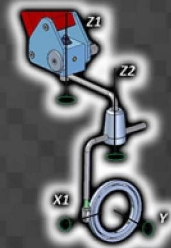
ORBITAL ATTACHMENT D FOR TOOLS FROM MIN \varnothing 60 MM TO \varnothing 85 MM
