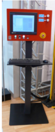
operating terminal with industrial panel PC and software i3stud (with DXF data converter)
